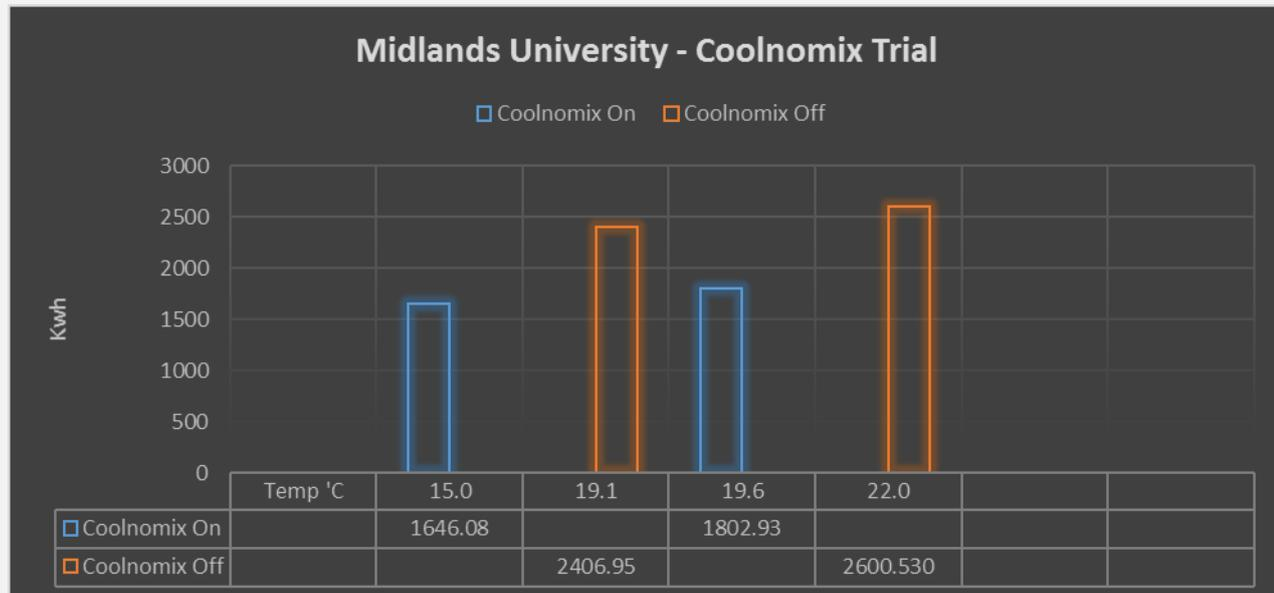
This is clearly shown, when comparing similar outside temperatures. The graph demonstrates that when the Coolnomix was not connected, the air conditioning unit was using **33.5%** more energy than when the Coolnomix was installed.
